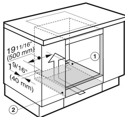
To ensure that the Combi Steam Oven has adequate ventilation, the following cut-outs measuring 19 11/16" x 1 9/16" (500 x 40 mm) must be made:
